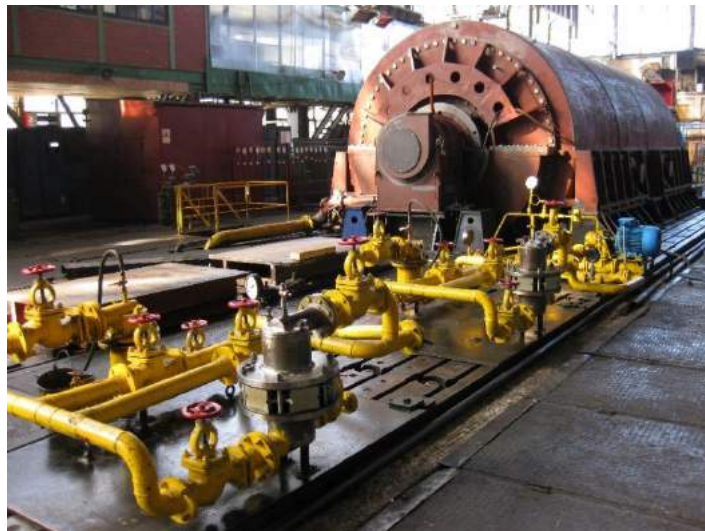
Figure 1. Turbogenerator type TGV-325-2AU3 on the factory test stand
